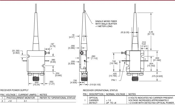
RF CONNECTOR: SMA (FEMALE STANDARD) OPTICAL CONNECTOR: FC/APC STANDARD (OTHÉR STANDARDS AVAILABLE)
