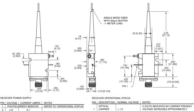
1.3 V/mW WITH DETECTED OPTICAL POWER UP TO +8 DETECT RF CONNECTOR: SMA (FEMALE STANDARD)
