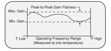
The gain flatness of a fiber link is measured by viewing the swept gain and determining the difference between the minimum gain and the maximum gain recorded over the operating frequency range. Unless the fiber link is specified to operate over a defined temperature range, this measurement is performed at room ambient temperature (+23°C). If a range of temperatures is specified, the measurement must also be verified at the temperature extremes.
